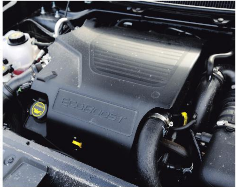
The Flex lineup starts with a standard 3.5-litre 287-hp TI-VCT V6 engine but, tested here, the Limited model ups the power ante with a 365-hp 3.5-litre twin turbo EcoBoost V6 mated to a SelectShift six-speed automatic and all-wheel-drive (AWD).
