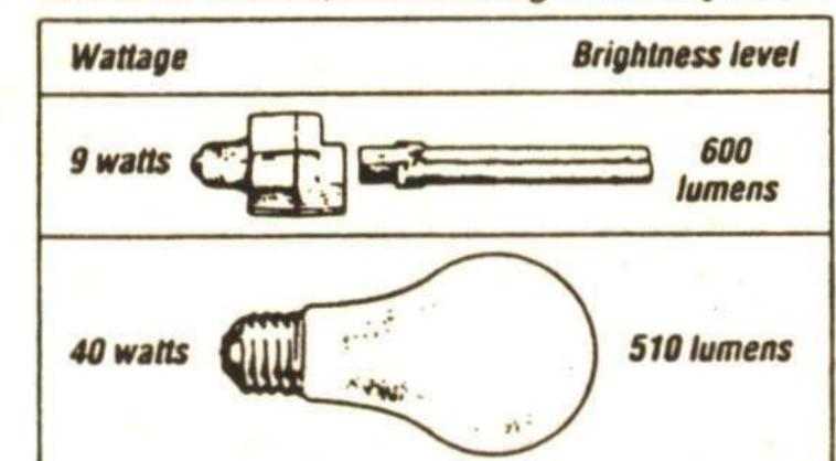
A 9 watt compact fluorescent, top, uses 78% less electricity and produces more light than a 40 watt incandescent bulb.
