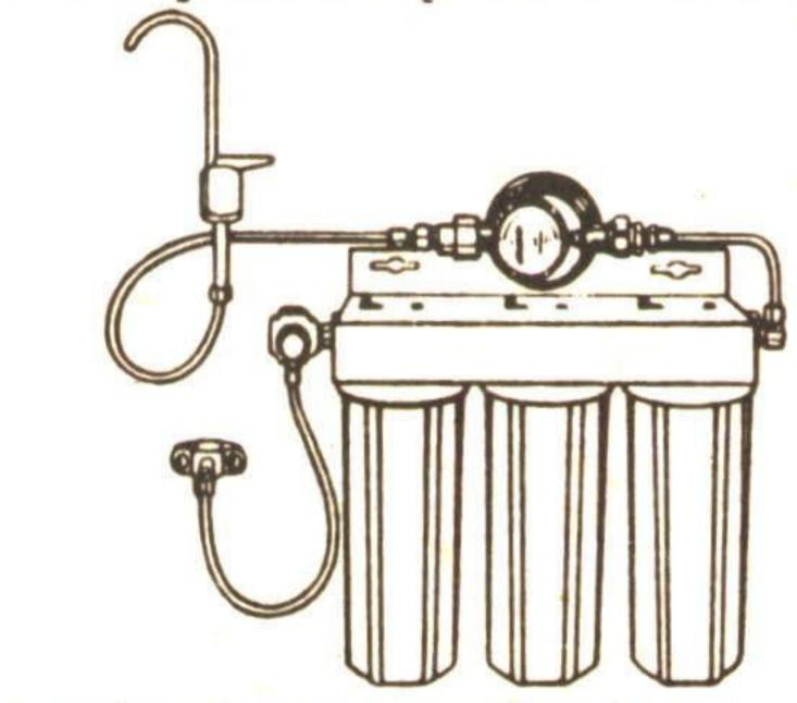
Granular activated carbon absorption is an accepted method of removing chemical contaminants from drinking water, particularly at the point of use. However, the flowing water must be in contact with the carbon for a prescribed length of time to be effective. To accomplish this, Ametek's system includes a pressure regulator and flow controller to provide more than enough contact time as water flows through the twin carbon cartridges.
