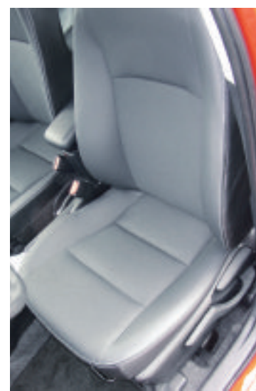
Part of the Premium Package option are seats trimmed with SofTex that is half the weight of leather and gives off just one per cent of emissions during manufacturing.
