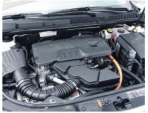
In the eAssist version of the 2012 Buick LaCrosse, the standard V6 is replaced by a 2.4-litre Ecotec four-cylinder with 15 kW electric motor/generator for a combined 182 hp and 172 lb/ft of torque.
