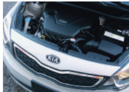
A 1.6-litre inline four-cylinder engine featuring gasoline direct injection powers the new Kia Rio sedan. Driving the front wheels, it produces 138 hp and 123 lb/ft of torque.
