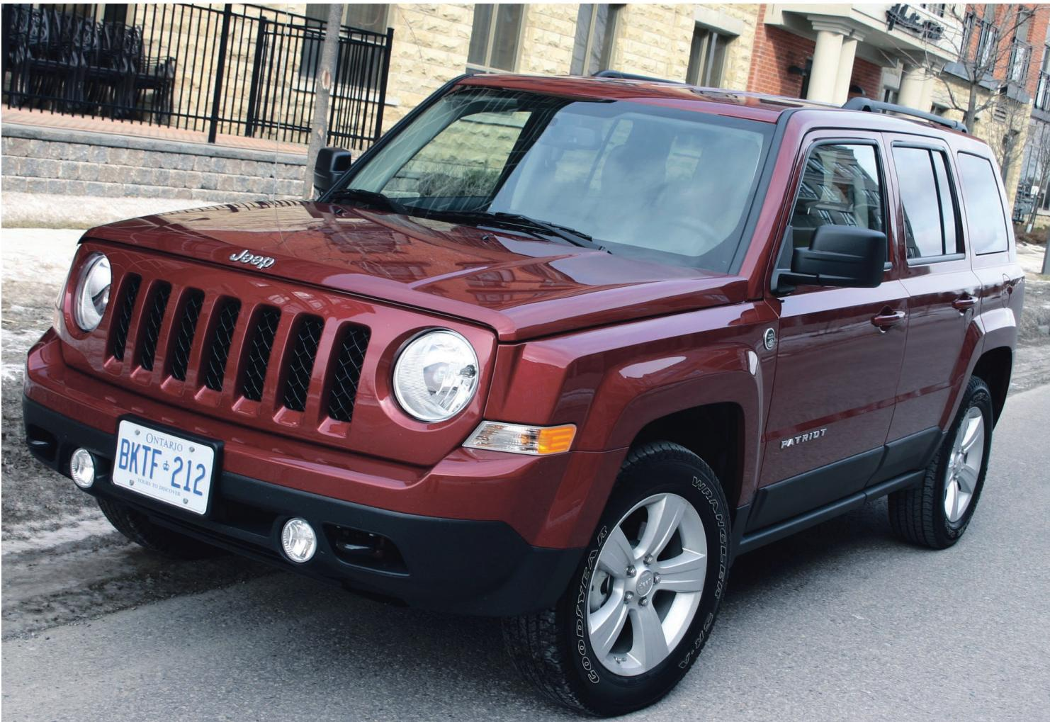
More rugged looking than its Compass sibling, the Jeep Patriot includes essential elements like the seven-slot Jeep grille, along with true off-road capability. As tested, this 'trail rated' Patriot includes tow hooks front and back, skid plates and a full nine inches of ground clearance.
