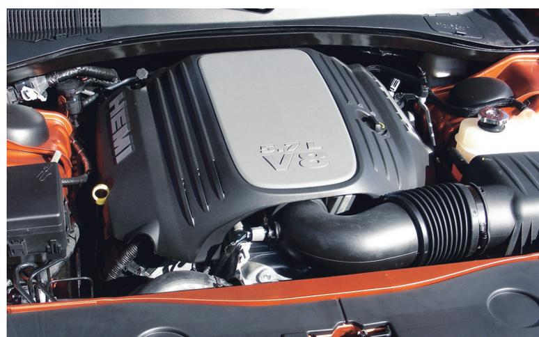
Yes, it has a Hemi with 372 hp and 401 lb/ft of torque (shown) but the 2011 Dodge Charger also offers a variable valve timing 3.6-litre V6 producing 292 hp and 260 lb/ft of torque.
