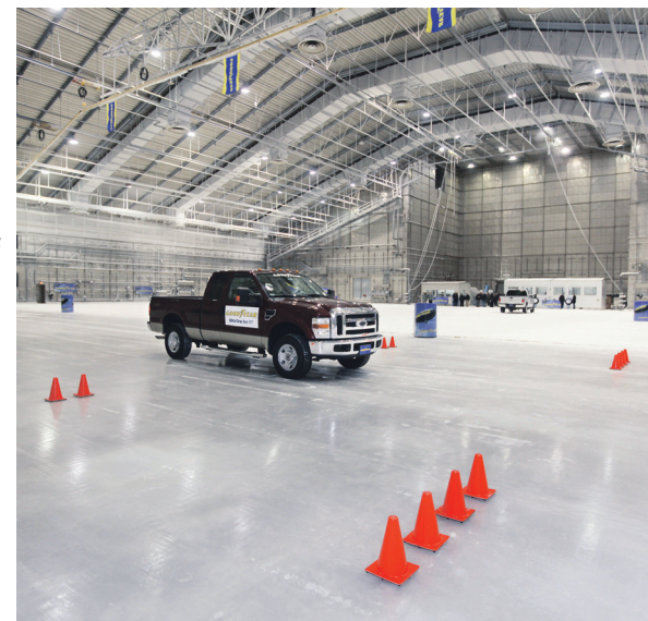
Winter tire testing in Florida, inside the McKinley Climatic Laboratory, an immense scientific building that can hold a 747 and test temperatures ranging from -65F to +165F. The building is located within the gates of Eglin Air Force Base in Florida.
