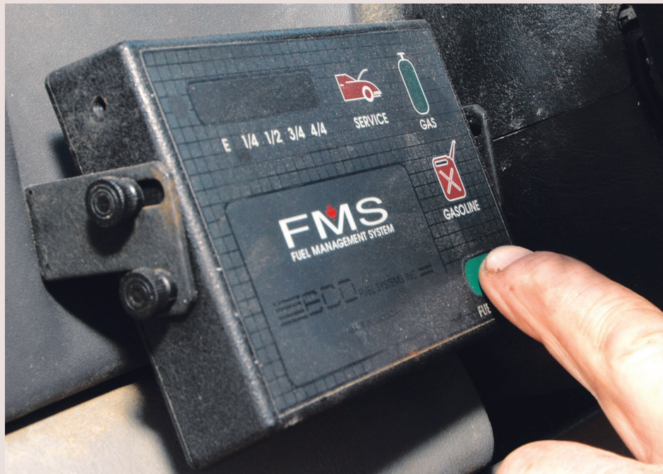
With the simple push of a button, Gordon can switch from gas consumption to NH3 on his Ford F350 pickup truck.
