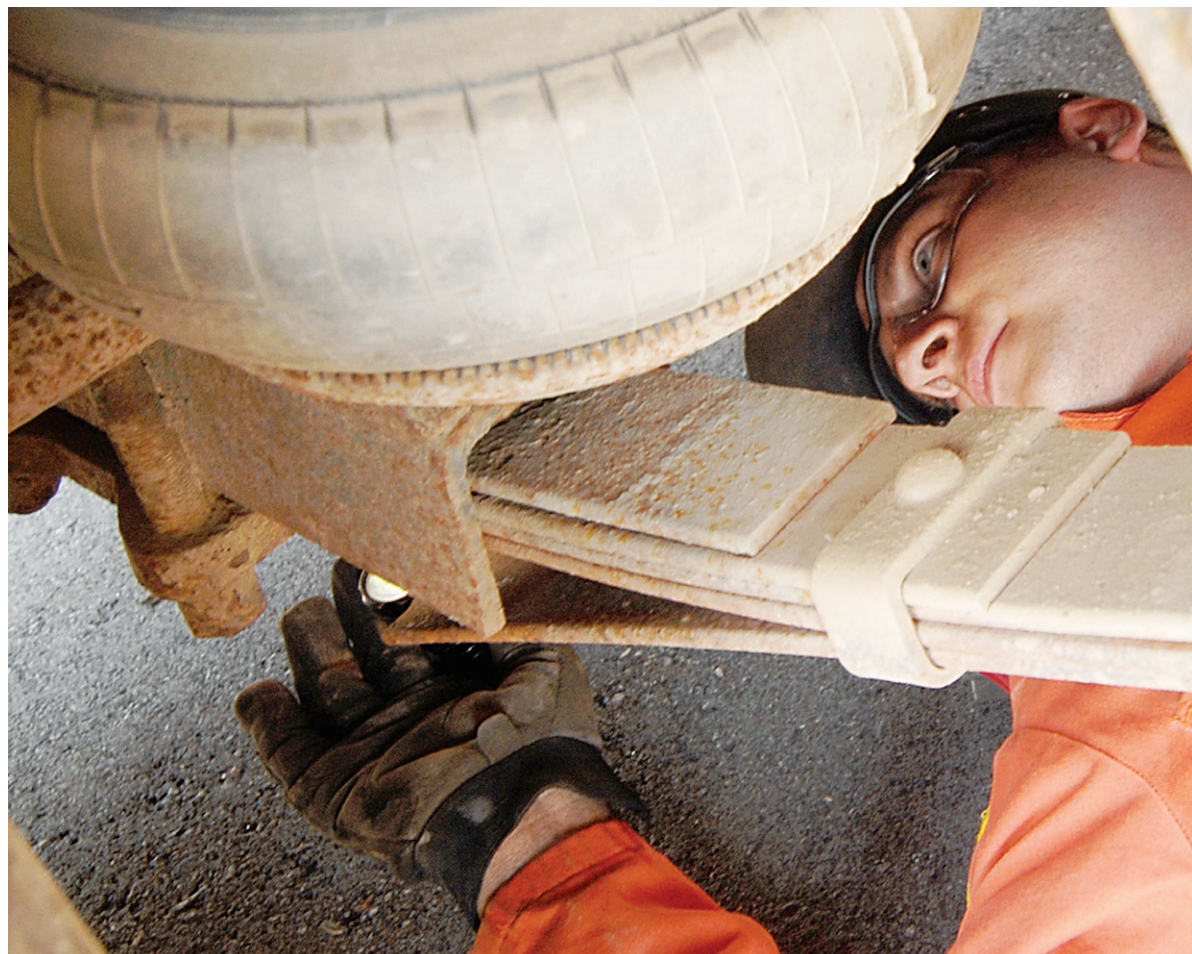
At a truck safety blitz in the parking lot behind Mold-Masters SportsPlex, Ministry of Transport Transportation Enforcement Officer Erik Eustace inspects a broken spring on a dump truck, one of the many pulled
