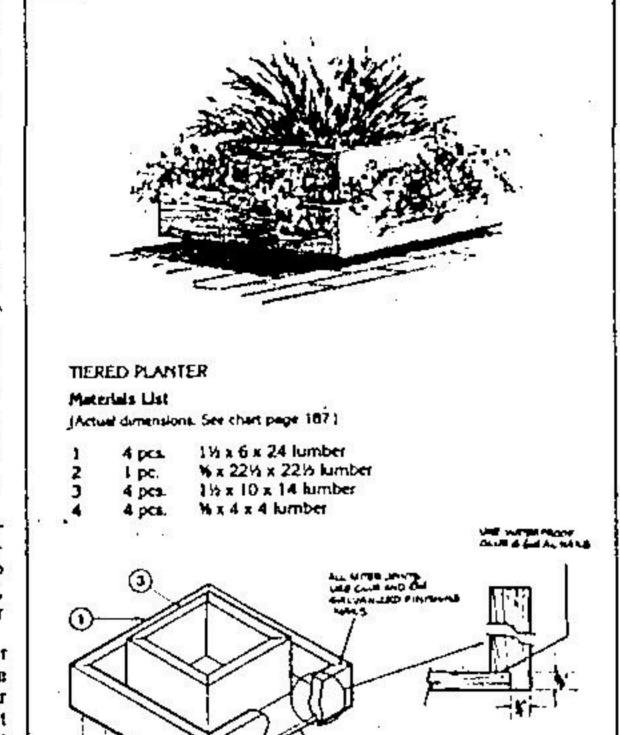
Use the right glue, reinforce with proper fasteners, then seal
