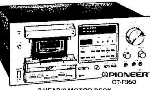
3 HEAD/2 MOTOR DECK Closed Loop Dual Capstan Drive Memory Stop/Repeat - Electronic Controls 20-19000; 0.04% Wrms, S/N 69DB
