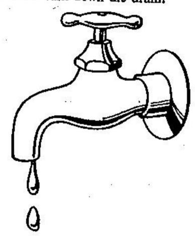
The compression tap is the most common type found in Canadian homes. The flow of water is regulated by turning a handle which is attached to a threaded spindle. When the spindle is turned down, the washer or disc attached to the bottom of the spindle is pressed tightly against a smoothly finished rins or ground seal to shut off the flow of water.
