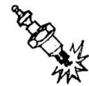
after 10,000 miles. B. The electrodes erode beyond the point of efficient functioning.
