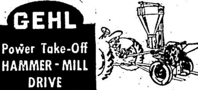
Come de and see this new Gehl engineering achievement. Now, the high efficiency of the famous Gehl Hammer Mill is stepped up even higher with Power Take-Off from tractor. It increases capacity of the mill as much as 50 per cent with the same power ... eliminates power loss caused by overly tight belts and belt slippage.
