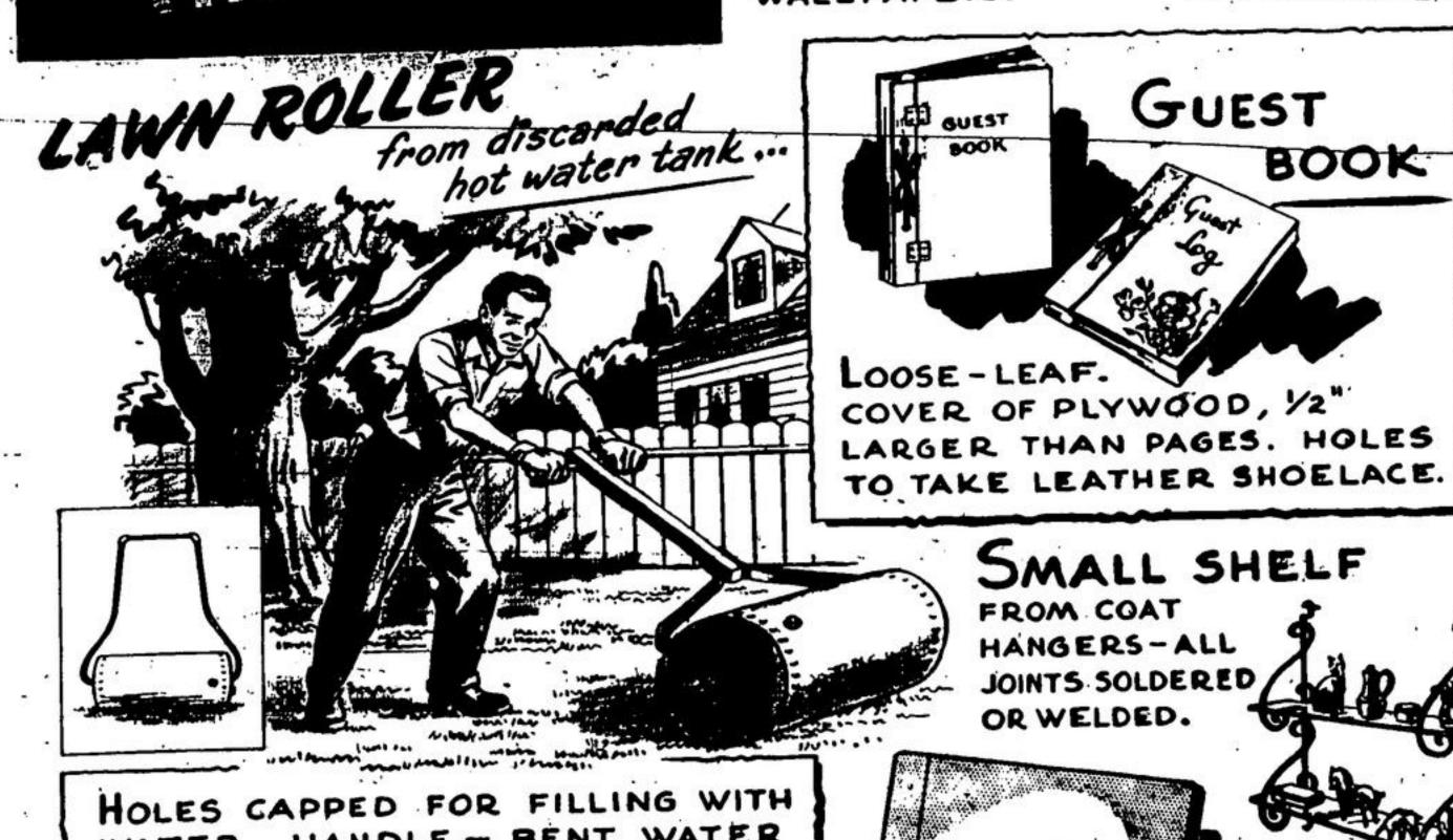
WATER. HANDLE - BENT WATER PIPE, FASTENED WITH ELBOW COUPLINGS ... OR 2x2, WITH TWO PIECES FROM DISCARDED WAGON OR CAR SPRINGS, FASTENED WITH BOLTS.
