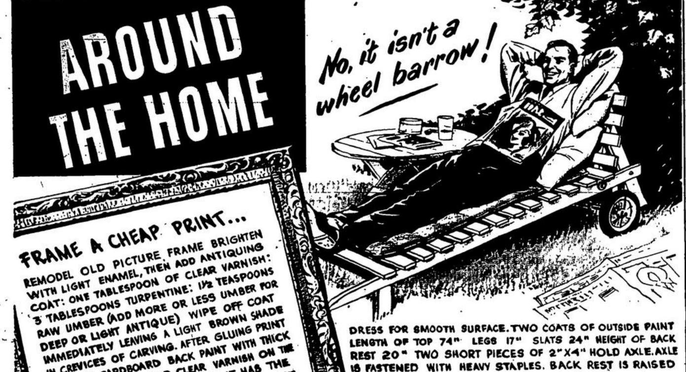
DRESS FOR SMOOTH SURFACE. TWO COATS OF OUTSIDE PAINT LENGTH OF TOP 74" LEGS 17" SLATS 24" HEIGHT OF BACK REST 20" TWO SHORT PIECES OF 2"X4" HOLD AXLE.AXLE IS FASTENED WITH HEAVY STAPLES. BACK REST IS RAISED OR LOWERED BY NOTCHED PAIR OF SUPPORTS.
