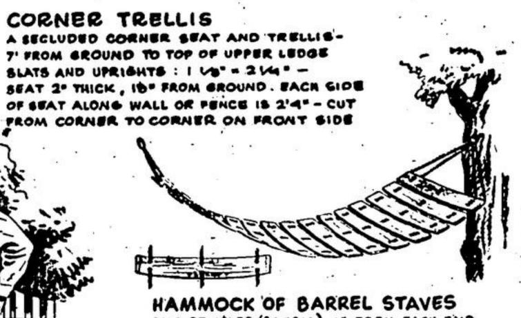
PAIR OF HOLES (%4"DIA) I" FROM EACH END AND AT CENTRE OF STAVES. WE ROPE THREADED DOWN ONE HOLE AND UP THE CTYIR. STAVES LEFT I APART. FASTEN UNDS OF ROPE TO LARGE RING OR BLOCK.
