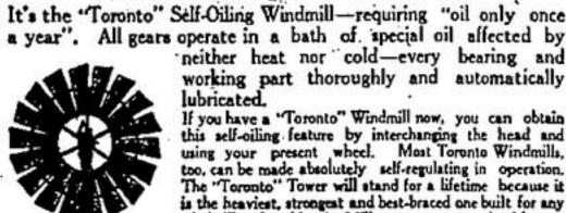
a year". All gears operate in a bath of special oil affected by neither heat nor cold-every bearing and working part thoroughly and automatically If you have a "Toronto" Windmill now, you can obtain this self-oiling feature by interchanging the head and using your present wheel. Most Toronto Windmills, too, can be made absolutely self-regulating in operation. The "Toronto" Tower will stand for a lifetime because it
