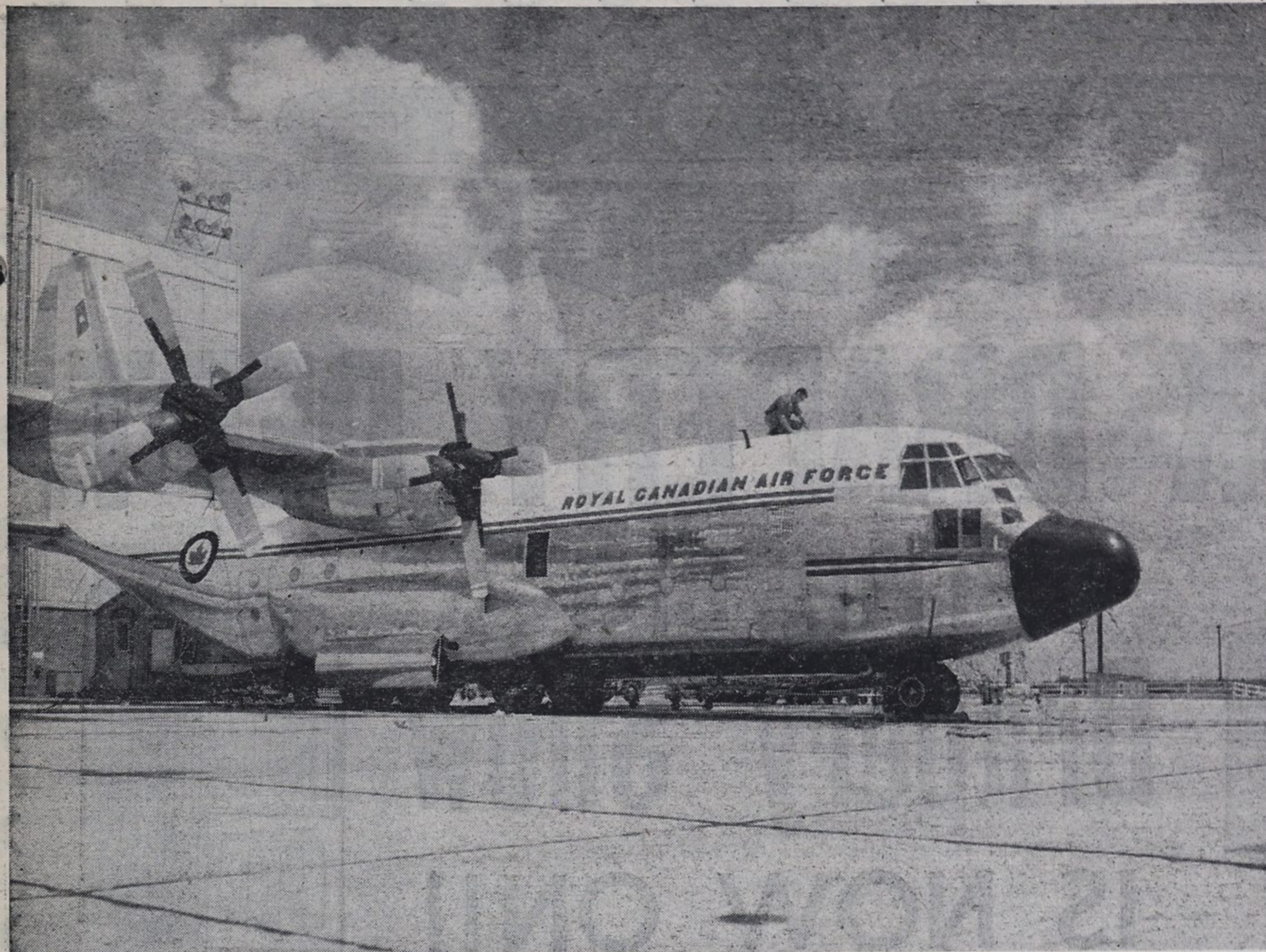
Just off the Lockheed Aircraft production line, is the first of the RCAF Hercules four engine turbo-prop jet heavy transport aircraft. Featuring easy manoeuvrability and rapid loading facilities, the 60 ton giant airlifter can be converted to carry 92 airborne troops or 15 tons of cargo and land them in remote sections of the world, in sandy deserts or arctic ice fields, with a non-stop range of 3400 miles. The first Hercules is expected to be in service with the RCAF later this year.
