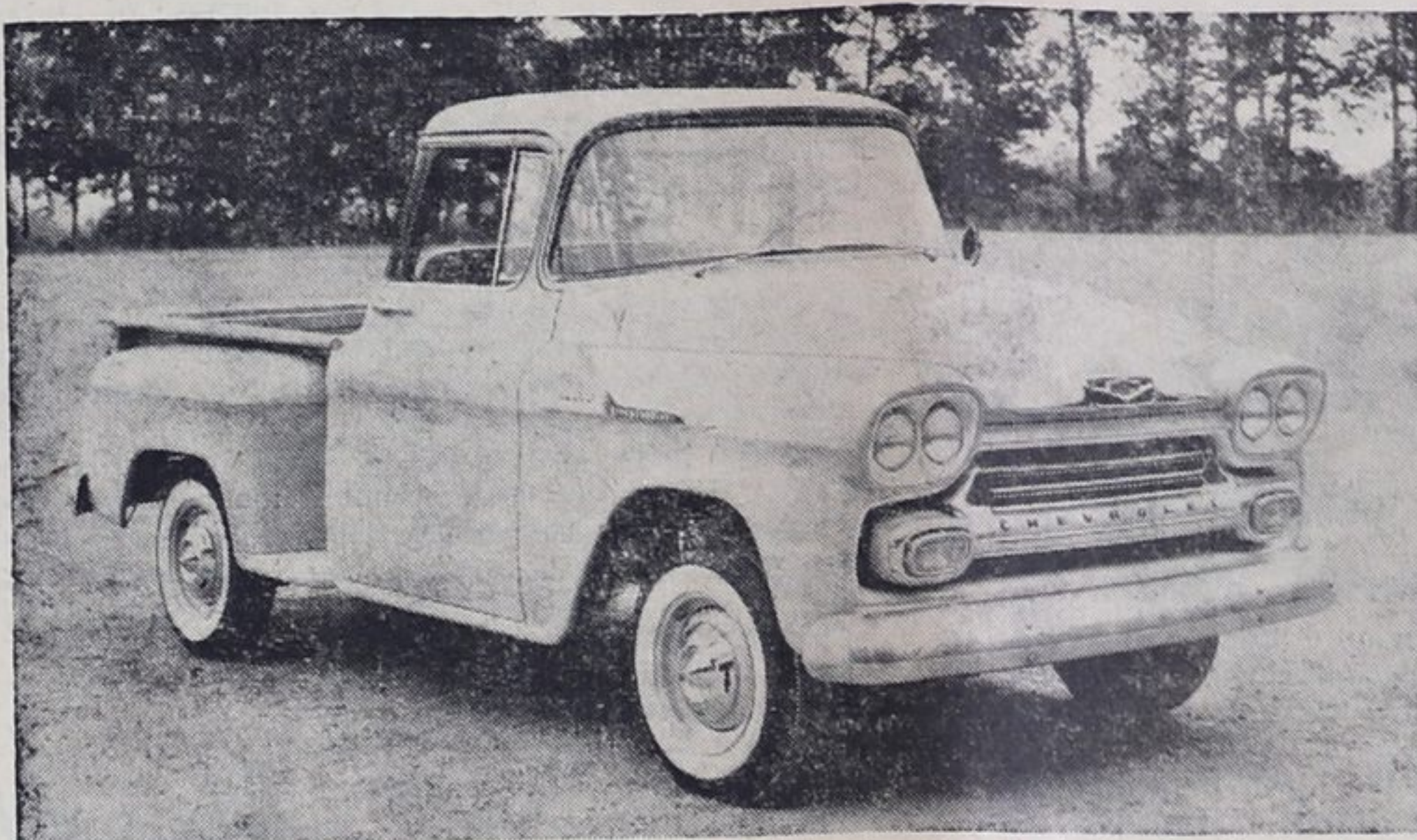
With fresh new front-end styling, including dual headlamps and redesigned grille, hood, and fenders, the 1958 Chevrolet Apache light-duty pickup truck packs more power in its 235 cu. in., 145 hp. six cylinder engine. Chevrolet's 283 cu. in. V8 rated at 160 hp., is available as an option. Also offered as optional equipment are Hydramatic or four-speed heavy-duty transmissions. The straight sides and floor with full width tailgate of the grain-tight box make shovel operations easy. It also permits uniform loading of drums, cartons and other containers.
