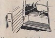
**New concealed Safety Steps** Running boards are ancient history now. Chevrolet's new Safety Steps are out of sight with the doors closed. That way, snow, ice or mud can't collect to cause accidents. Safety Steps are lower, too, for easier entrance.
