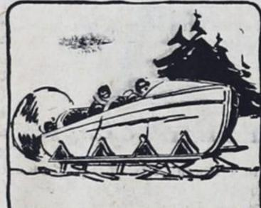
THIS SELF-PROPELLED SLED, POWERED BY A PROPELLOR AT THE BACK WAS SAID TO DO 60 MPH. IT WAS SHOWN IN A BERLIN AUTO SHOW WAY BACK IN 1912.
