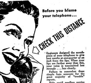
Engineers designed the mouth-piece of your telephone to give best results at one-quarter of an inch from the lips. When your lips are farther away than this, your voice is transmitted less strongly...less clearly.
