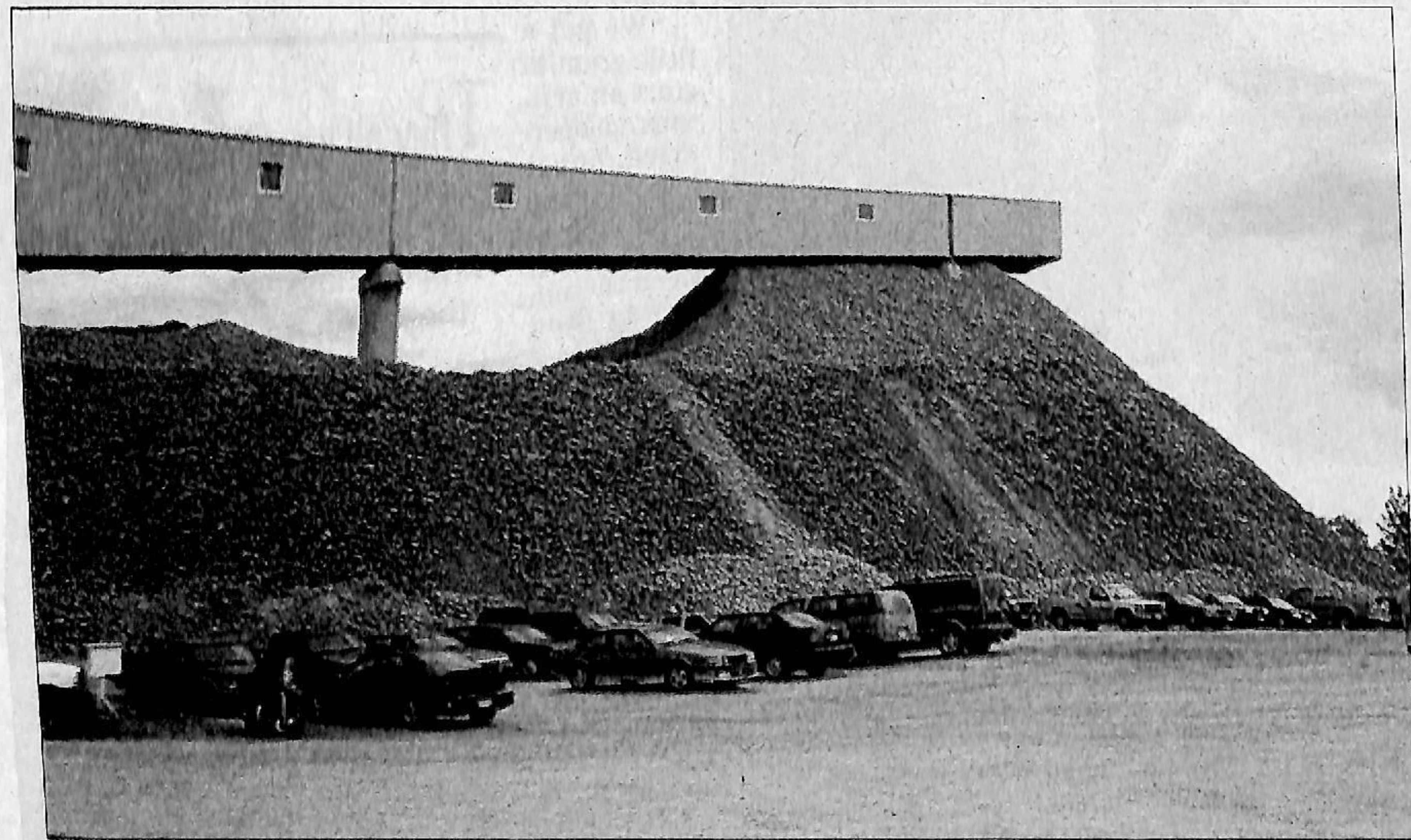
It's a long way to Lake Ontario from the Ogden Point Quarry so the ore is carried by conveyer to the James Norris awaiting at the pier.
