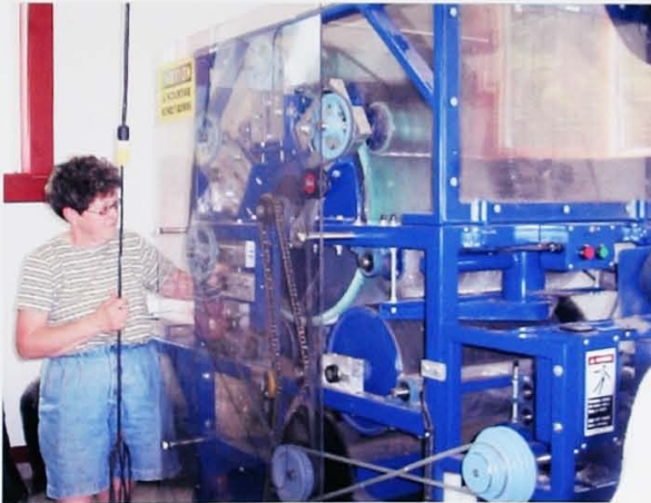
Draw frame - stretches the fibre more.
