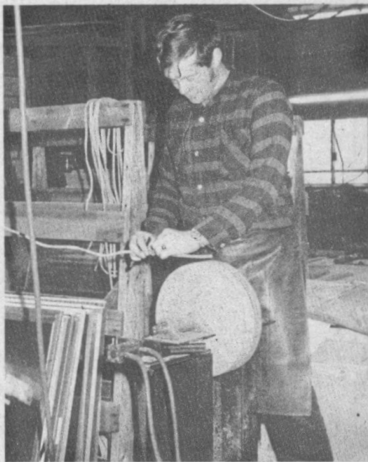
DAVID FLEMING, cutting a strip for an aluminum sash.
