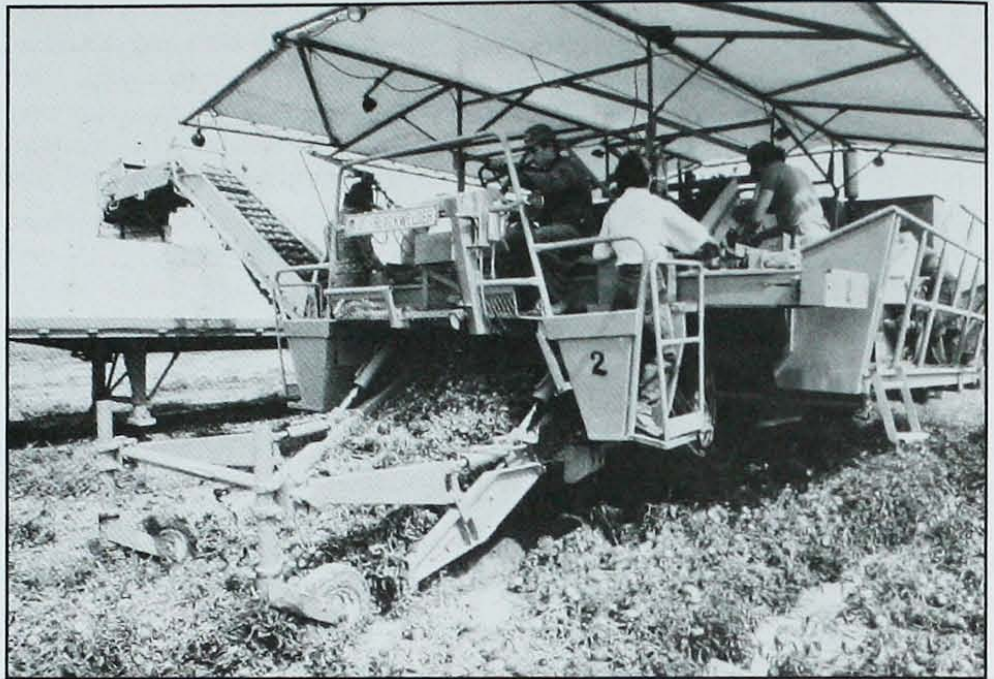
A tomato harvesting machine showing the tomatoes coming up from the field on a conveyer belt. Photo courtesy of the OMAF Film Library
