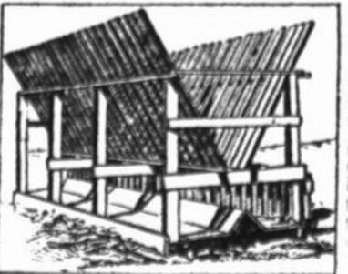
The runners are 2 by 6, the framework of 2 by 4, and the slats forming the "V" trough are 1 by 4. The plan clearly shows how to make this feed rack.—Farmers Mail and Breeze.
