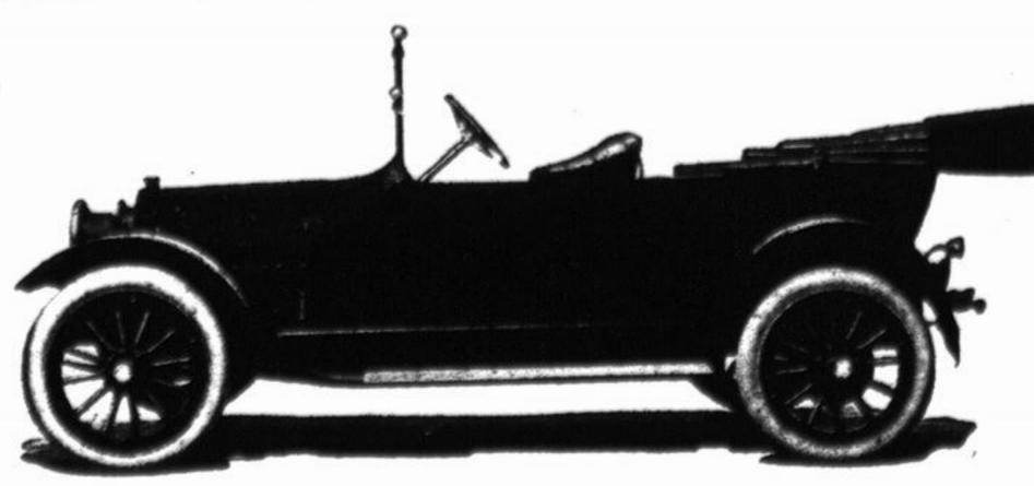
Left side drive, and center control. Access to all four doors. Electric starter and Electric Lights. One-man top and fully equipped without extra cost. 114 inch wheel base. Tires 33x4 inches front and rear. Crown fenders. Stream line Body. Splendid springs and abundance of power.
