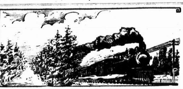
A fire line along a railway with two cleared spaces separated by a double row of trees intended to catch the sparks.
