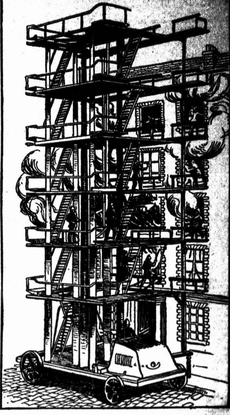
The rapid increase in the number of fatalities from fires in London has attracted the attention of inventors to the great problem of saving life endangered by fire and one result is the invention of a large motor car which carries a series of platforms with mechanical means for raising
