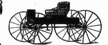
Gentlemen's High Grade Driving Wagon; 1 inch drop axle; body 22x56 glued, screwed and plugged; best hickory gear; broadcloth trimmings; patent wheels; I year guarantee.
