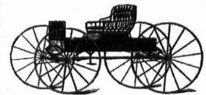
Gentlemen's High Grade Driving Wagon; i inch drop axle; body 22x56 glued, screwed and plugged; best hickory gear; broadcloth trimmings; patent wheels; I year guarantee.
