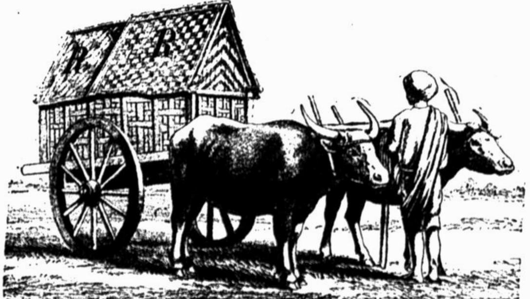
On this page we give an illustration of a Ceylonese team of buffaloes hitched to a cart common to that country. It will be noticed that the tongue is fastened to a yoke bound to the horns. Thus the weight of the pull is on the horns and not on the shoulders, as with
