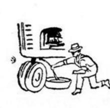
First, either drain the radiator and block completely, or fill with the correct amount of anti-freeze. If storing for very long periods, also drain the entire fuel system, fuel tank, settling cup, fuel lines, screens and carburetor. Remember, fuel left in the tractor for a long period of time
