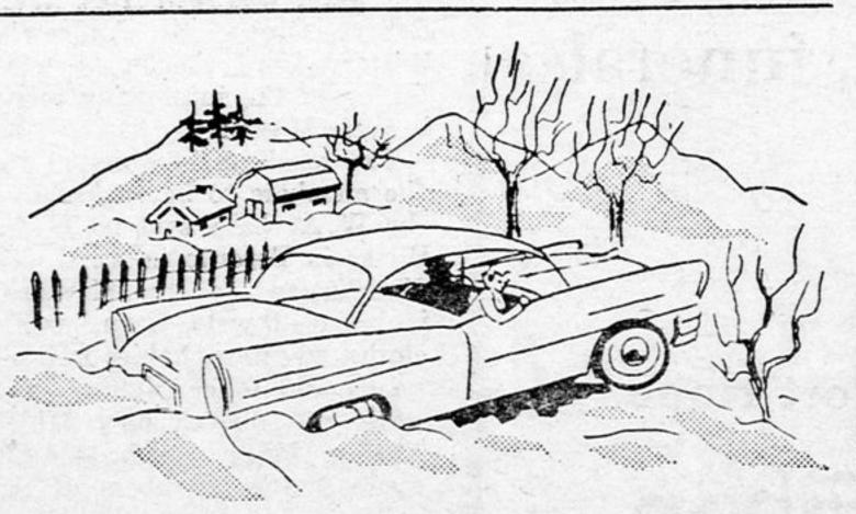
GETTING OUT - WHEN YOU'RE STUCK - Start slowly forward in low gear. When you have moved as far forward as possible, shift to reverse. When the wheels spin, again shift to low. Repeat until car is free. Spinning wheels only digs you deeper into the snow.
