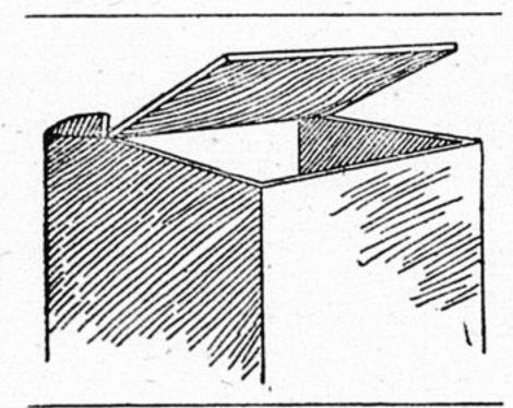
some device that will not let the covers open past the perpendicular line—compelling one to hold it open while he dips out the grain. Such a device is shown in the sketch. Such a "stop" should be nailed upon either end of the box. The same end can be secured, if the cover opens back against a wall, by nailing a piece of board to the wall, that will keep the cover from coming back past the perpendicular.
