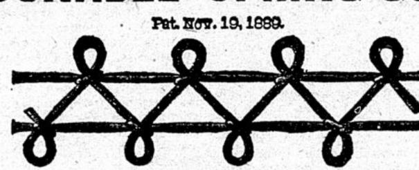
Above Cut is One-half Actual Size. Most Attractive in Design, and will stand a Test Breakage of 2,500 lbs.
