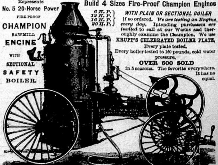
The sectional safety botter is manufactured expressly for the 'North West" trade. This boiler is so arranged that it is readily taken apart in sections enabling purchasers to clean thoroughly every part of it and prevent burning out We know from experience this is absolutely necessary with the alkaline waters of the great Western prairies. Largely used by the Pacific Railway Company and all the large Colo-
