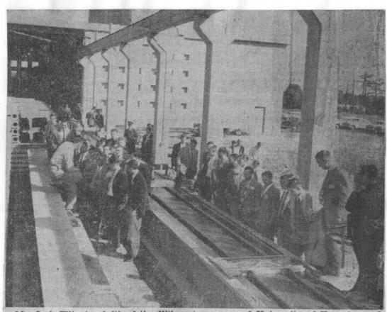
Mr. Jack Ellis (on left) of the Wilson | a group of University of Toronto grad-Concrete Products Ltd. is explaining the procedure of preparing the mould for pouring a pre-stressed concrete beam to | Wilson plant yesterday afternoon.
