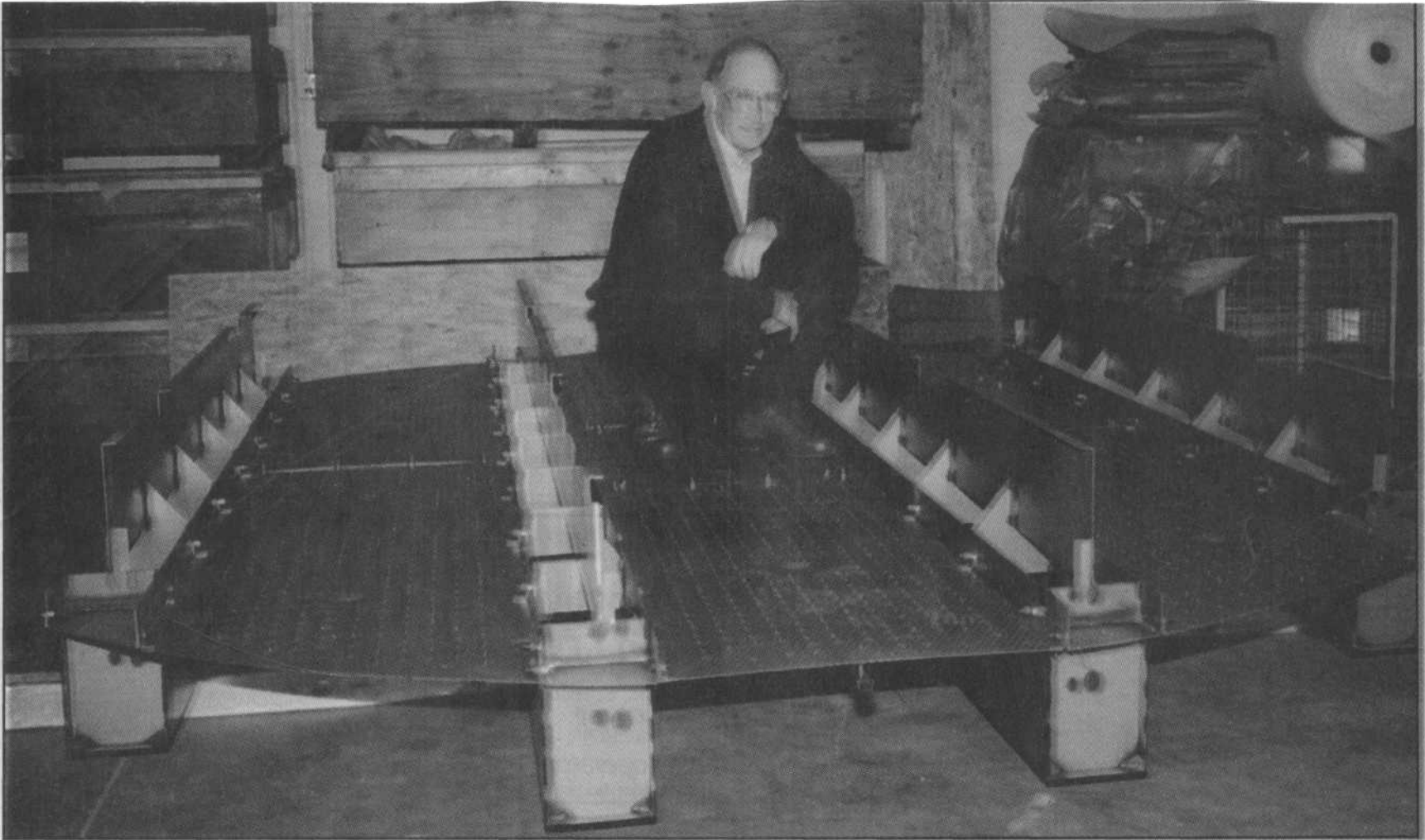
Quest-Tech Precision Inc. general manager Peter Savidge is with one of the large petrochemical refining trays that the company produces at its Jamieson Bone Road facility.
