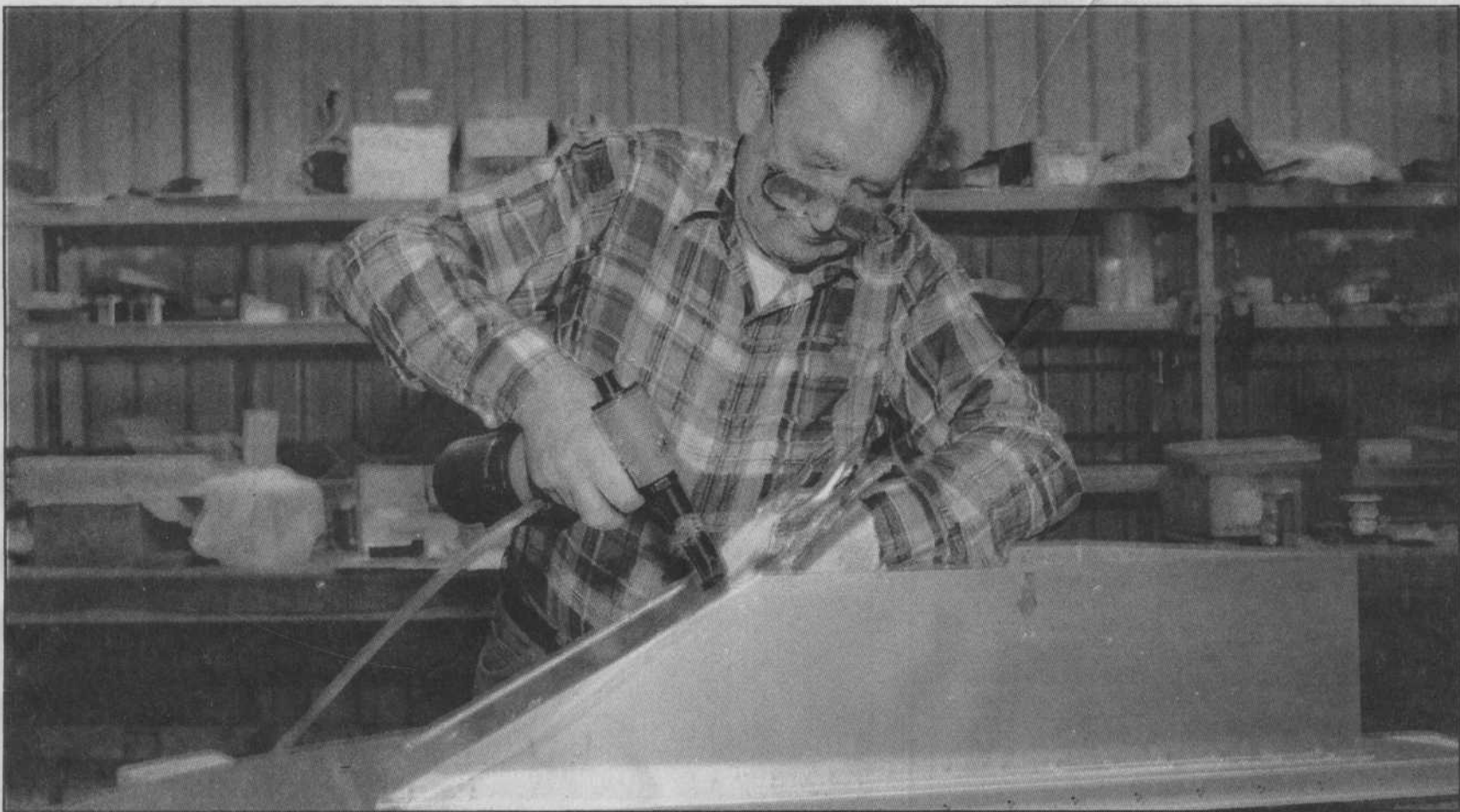
Quest-Tech Precision employee Bill Attwells assembles an air separation tray for a gas separation plant.
