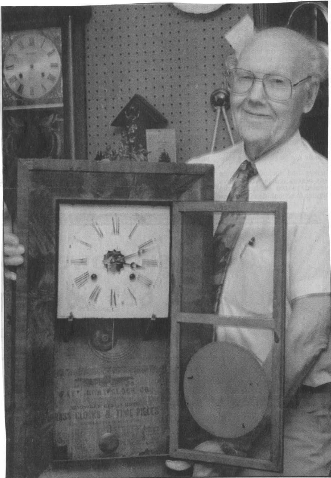
Intelligencer photo by Jennifer Be Watchmaker Al Reid of The Time Zone Jewellers is repairing a 150-year-old Waterbury clock made in Connecticut, one of thousands of such clocks that sold for approximately $4 US in the mid-19th century.
