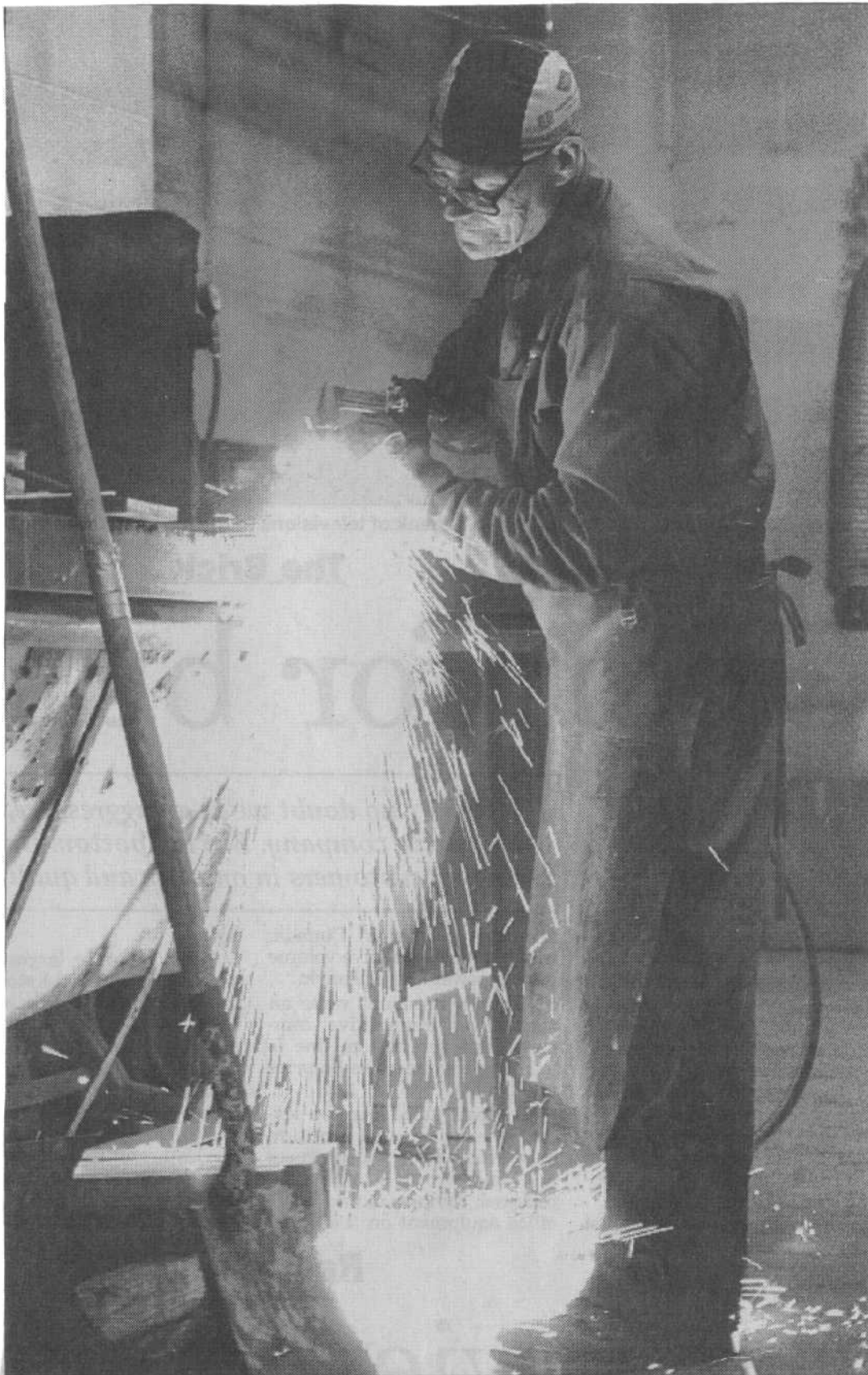
Pre-Con's Mike Hogan alters metal forms used to contain the wet concrete. The plant has its own metal fabrication and welding shop.
