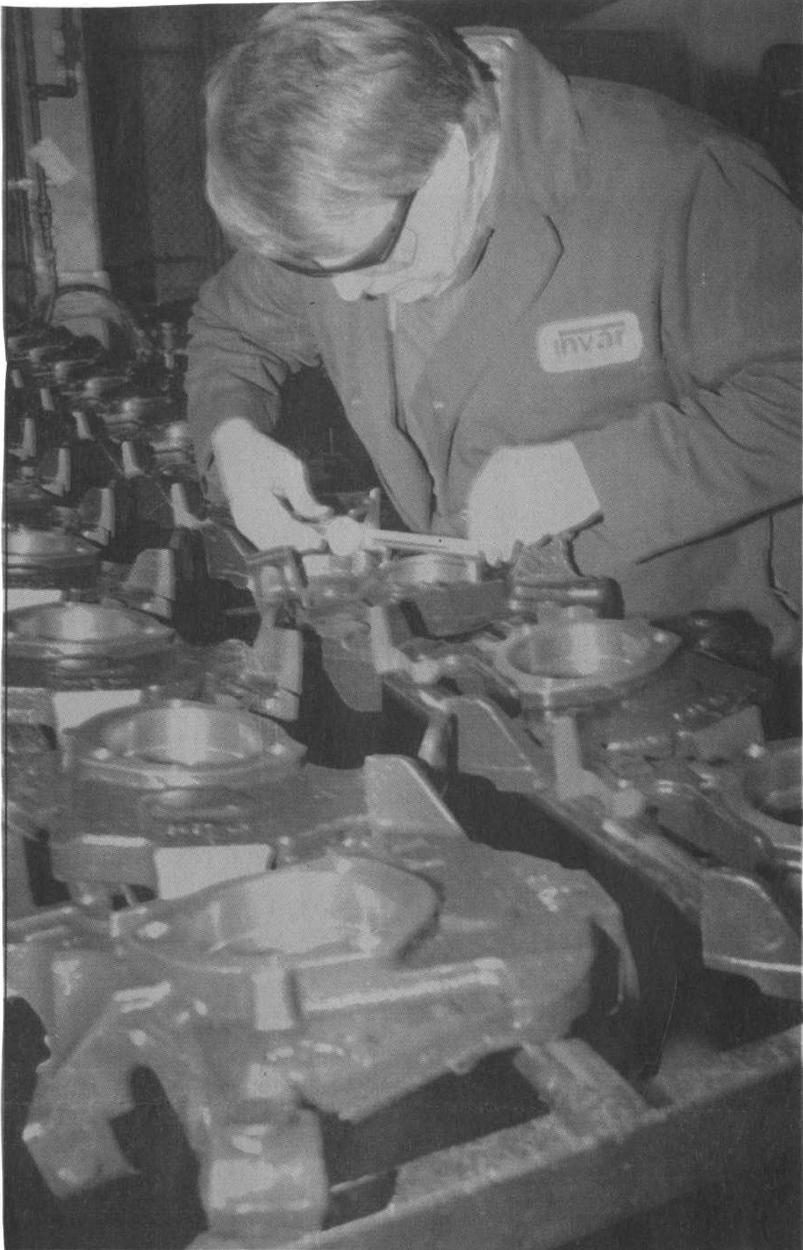
Ray Gorse, horizontal mill operator at Invar Manufacturing, inspects a row of completed "knuckles", a cast-iron machined component made for General Motors' Tahoe and Suburban truck lines.
