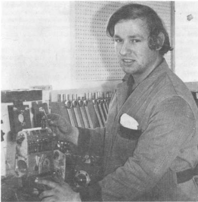
Danny Sagriff, a first year trainee at Diesel Injection Service, is shown disassembling a fuel injection pump off an International B250 farm tractor.
