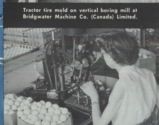
Golf ball stamping machine at A. G. Spalding & Bros. of Canada Limited.
