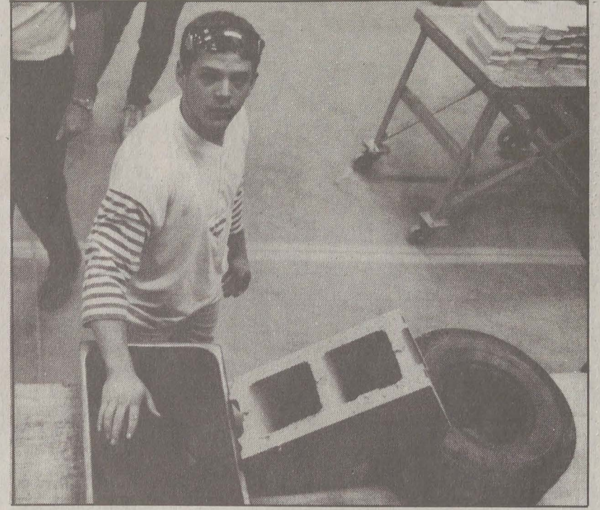
Billy Vogt, second year Concrete Technology student, sifts a handful of ground-up rubber, the raw material of a new project to test the use of waste rubber tires as an ingredient in concrete blocks. Block pictured above is one of the first samples of this new technology.
